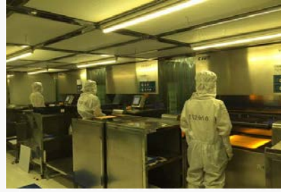
Sheet by sheet exposure Class 100 clean room
