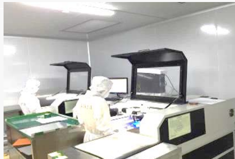
Laser/die cutting Tolerance control: +/-0.15mm
